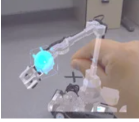
(a) Controlling robot arm using a virtual sphere. Robot displays hologram of target position.
